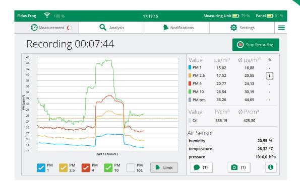
Fig. 3: Display of measured values during a measurement
