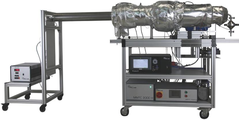
In this version, the filter holder MMTC 2000 E is made of V2A in order to cover a higher temperature range. The addition of heating and insulation allows filter testing at temperatures of up to 250 °C.
