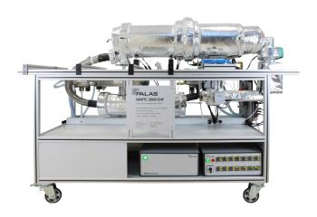
In this version, the filter holder MMTC 2000 EHF is made of V2A to cover a higher temperature range. Adding heating and insulation allows filter testing at temperatures up to  $250\,^{\circ}$ C.
