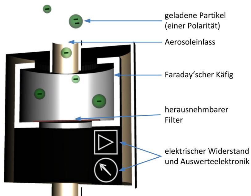
Fig. 1: Principle of operation of the Charme<sup>®</sup> aerosol electrometer
