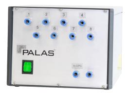
The Muti Sampling System MSS 08 enables the connection of central measuring devices (e.g.,  $UF-CPC^1$  or  $ENVI-CPC^2$ ) up to eight different sampling ports and easy switching between them. This can be useful, e.g., for nanoparticle concentration monitoring in different rooms or along a process with a single measuring device.
