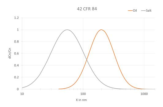
Based on the measurement of particle penetration via particle size, the PMFT  $1000 \, \text{F}$  can also be used to consider the tolerances in the particle size distribution according to EN 13274-7 as a min. / max. penetration value.
