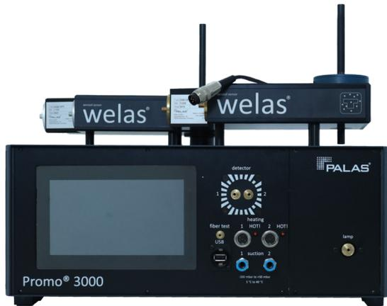
The welas<sup>®</sup> aerosol sensors welas<sup>®</sup> 2070 HP, 2100 HP, 2200 HP, 2300 HP, and welas<sup>®</sup> 2500 HP are equipped with a cuvette heatable up to 120 °C and pressure-tight up to 10 barg to ensure isobaric and isothermal sampling into the sensor's measurement volume.
