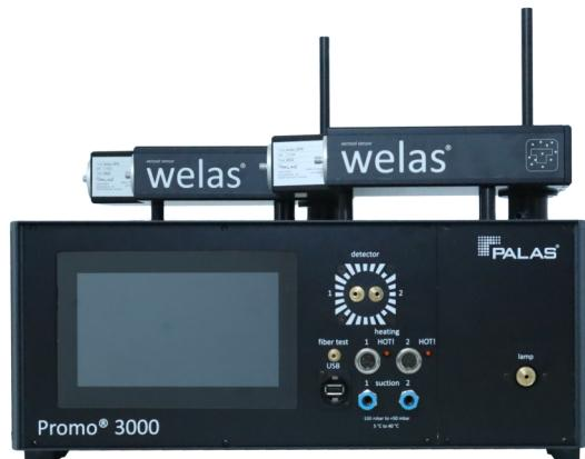
The welas® aerosol sensors welas® 2070 P, 2100 P, 2200 P, 2300 P, and welas® 2500 P are equipped with a pressure-tight cuvette to ensure isobaric and isothermal sampling into the sensor's measurement volume.
