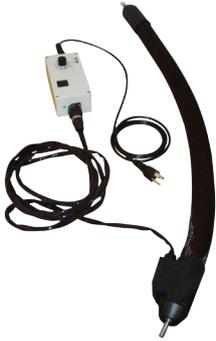
The sampling tubes PS 1000 / PS 2000 and PS 3000 can be heated up to 120 °C and easily adapted to the heated welas® aerosol sensors. The heating control is part of the delivery content.
