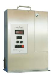
This device disperses particles at positive pressure values of up to 3 bar and can also use nitrogen and air as the dispersing gas. Optional operation with low pressure from 300 mbar absolute is possible. The 7-, 10-, 14- or 20-mm feed stock reservoirs are pressure-resistant. For operation with low pressure special pressure-resistant feed stock reservoirs are needed. Their piston is strongly connected to the feeding unit by a claw. This enables an undisturbed operation with low pressure.
