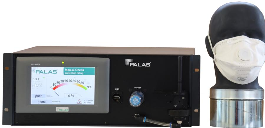
Palas® developed the Mas-Q-Check to subject protective masks to a quick, simple, and meaningful test before use. A particle-counting measurement device is used to detect efficiencies in the size range of viruses and bacteria. The system can also be used for training, as it immediately shows the efficiency of protective masks.
