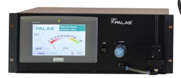
Palas<sup>®</sup> developed the Mas-Q-Check to subject protective masks to a quick, simple, and meaningful test before use. A particle-counting measurement device is used to detect efficiencies in the size range of viruses and bacteria. The system can also be used for training, as it immediately shows the efficiency of protective masks.
