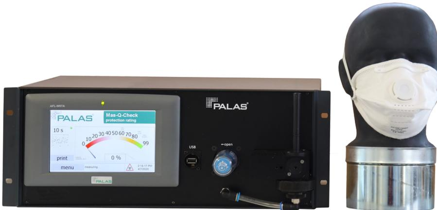
Palás® developed the Mas-Q-Check to subject protective masks to a quick, simple, and meaningful test before use. A particle-counting measurement device is used to detect efficiencies in the size range of viruses and bacteria. The system can also be used for training, as it immediately shows the efficiency of protective masks.
