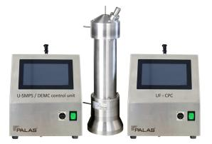
A soft X-ray source as a neutralizer is already integrated. The advantage instead of a radioactive neutralization (for example, with Kr-85) is that there is no need to follow requirements during transportation.
